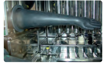
Leak tightness test
