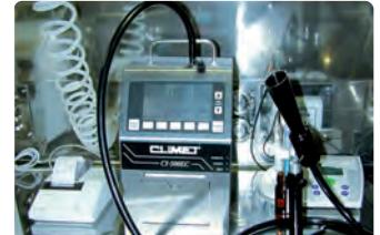
Particle Counting Test (Air classification)
