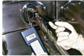
Laminar Flow Air Velocity
